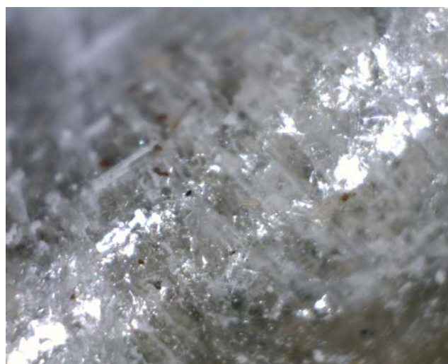
Fig. 4. Iron filings and pathways several layers deep into mica tape along top edge of top coil.
