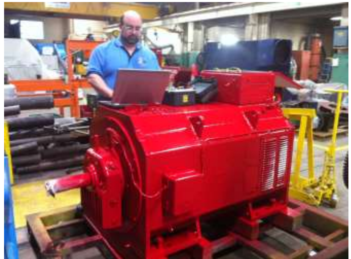
Figure 1. 1200kW Generator Under Test
